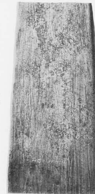
Longitudinal stone-saw marks on the reverse (flat) face of a Tlingit dagger blade of native copper. This photo has been made on ortho process film for maximum contrast in the topography of the cut surface; details of the cut and of crystal structure are thus exaggerated by photographic distortion. University Museum No. 42-30-42.
