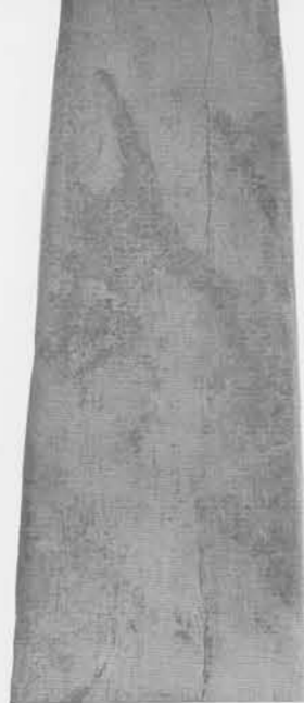
Portion of the faces of two Tlingit dagger blades of native copper, lighted and photographed so as to show the crystal structure of the metal as stained on the chelated surface. In our lighting, we were not entirely successful in eliminating the marks of the stone saw from our photographs. University Museum Nos. NA 1286, 42-30-42.
