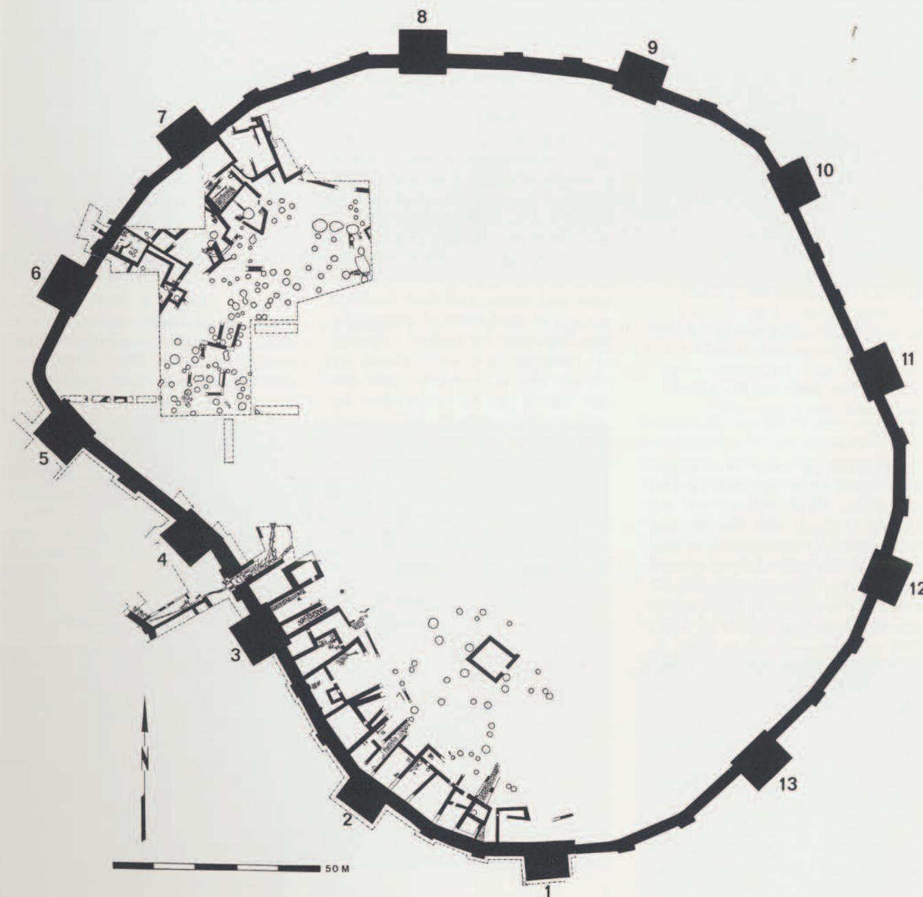
6 Preliminary plan of the Urartian citadel built in Hasanlu period IIIB. The nature of the settlement within the massive fortification wall is most clearly seen to the lower left. Small barracks-like rooms were built up against the wall, separated by narrow paved paths leading to great rectangular towers. In the open central part of the site were deep pits, presumably used for storage. (Drawn by the author)
