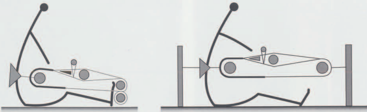
Fig. 10a, b. The Sobei use two simple loom types to weave terfo . (a) Termed Sobei type I, this loom employs the feet and back to maintain tension on the warp threads. (b) The Sobei type II loom uses poles placed in the ground at each end to keep the warps taut.
