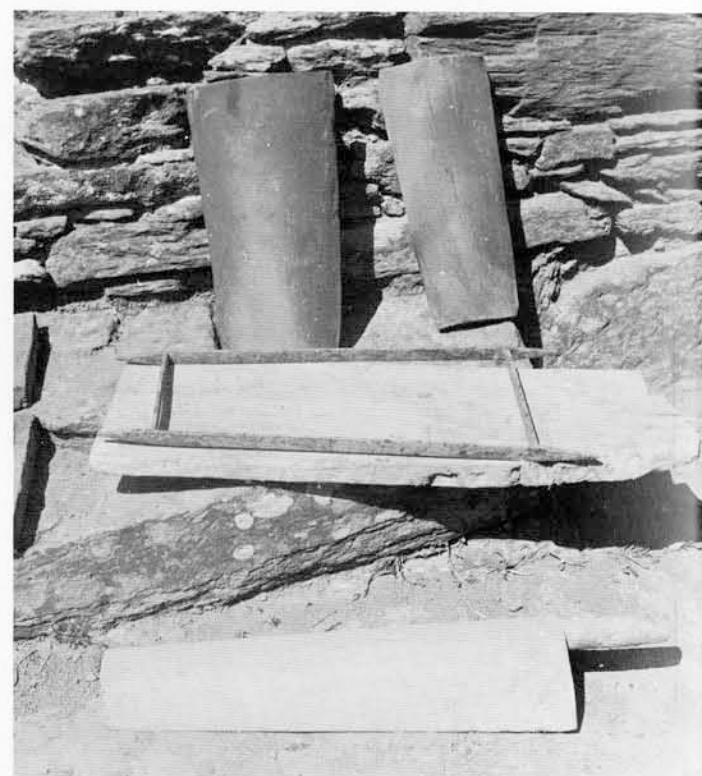
Tile-making equipment used by Kozanitis of Amolocho, to make the long curved and tapering tiles used in peasant houses. (A square frame for making mud-bricks can just be seen on the left hand edge of the picture.) The clay is rolled out to fill the iron frame on the flat wooden board, then flipped onto the curved wooden mold below. The tiles are sun-dried, then fired. They can be seen in the background.
