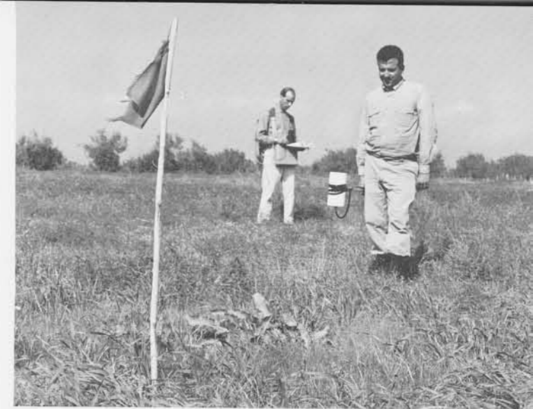
Varian Associates Precision Portable Cesium Magnetometer in use at Sybaris. Giacinto Loisi (foreground) carries cesium sensor and approaches end of grid line marked with flag. Franco Brancaleoni carries readout and batteries, and records readings in notebook.
