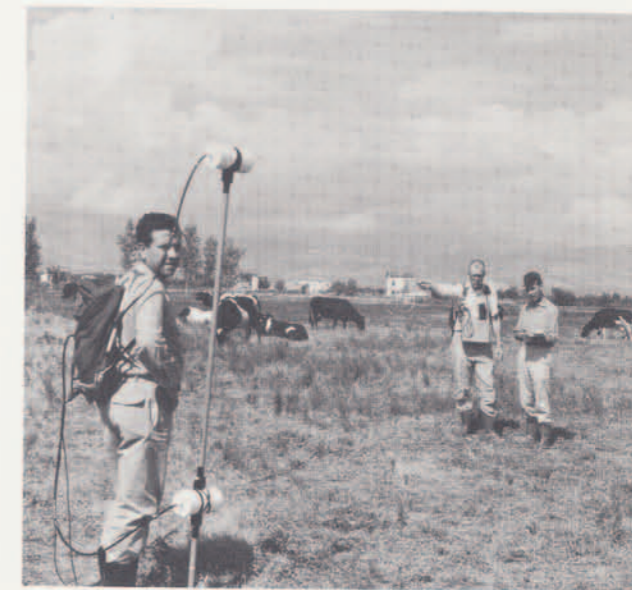
Cesium magnetometer in use in the Casa Bianca area, plain of Sybaris.
