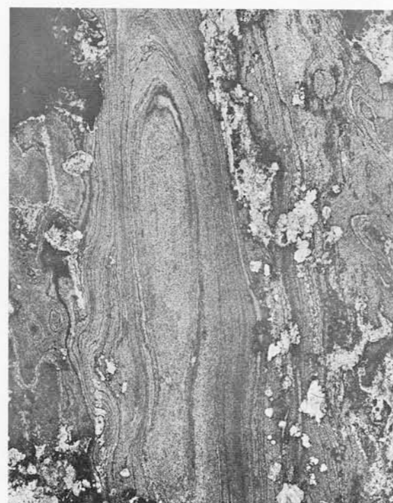
Photomicrograph of a steel spearhead of the sixth century B.C. from Deve Hüyük, Syria; the contorted piled structure indicates forging from a large number of carburized plates.
