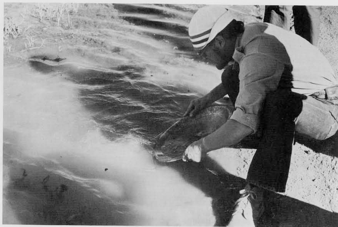
7 Mineralogist Fabian Cesbron (University of Paris VI) panning cassiterite sands in a qanat pool in the Sarkar Valley.
