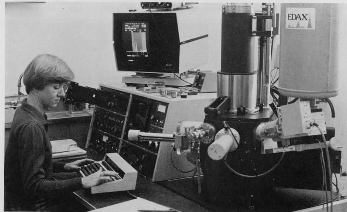
2 Deborah Ricketts, Research Specialist at the University of Pennsylvania's Laboratory for Research on the Structure of Matter (LRSM), is shown operating a Phillips 500 scanning electron microscope capable of 80,000x direct magnification. It is equipped with an ECON energy dispersive windowless spectrometer capable of detecting the presence of the traditional range of elements as well as a number of those with lower atomic numbers, including carbon, nitrogen, oxygen and fluorine. Photo courtesy of Alex Vaskelis and Robert White, LRSM.
