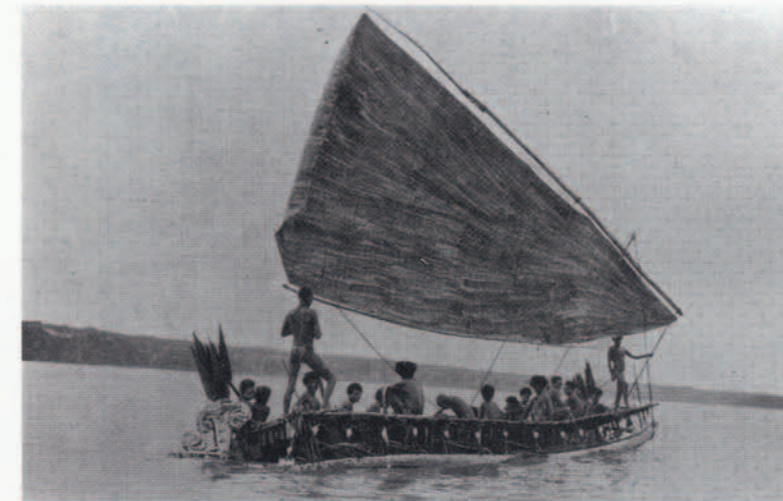
Fig. 2. Trobriands canoe under sail. These large, sea-going canoes are sailed with the wind coming over the outrigger side, so that when the canoe tilts, the outrigger float rises. To sail with the wind coming from the opposite quarter, the mast of a canoe like the one illustrated here must be unstepped from one end of the hull and resteped at the other, thereby reversing the bow and stern. For this reason, the canoe has "prow" boards at both ends.
