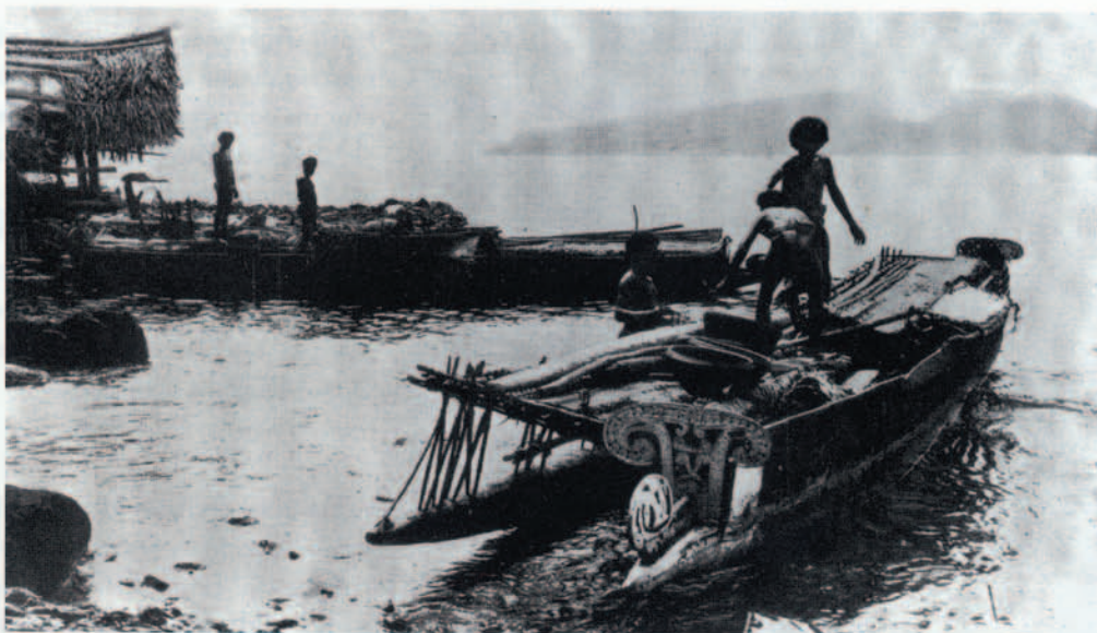
Fig. 3. Trobriands trading canoe. At the ends of the canoe, transverse prow-boards close off the longitudinal planking that raises the sides of the dugout hull. Other oval-shaped boards project from them at right angles. The space between the dugout hull and the outrigger float is spanned by a platform on which cargo is carried. This Trobriands canoe is being loaded with large clay pots from the Amphlett Islands.
