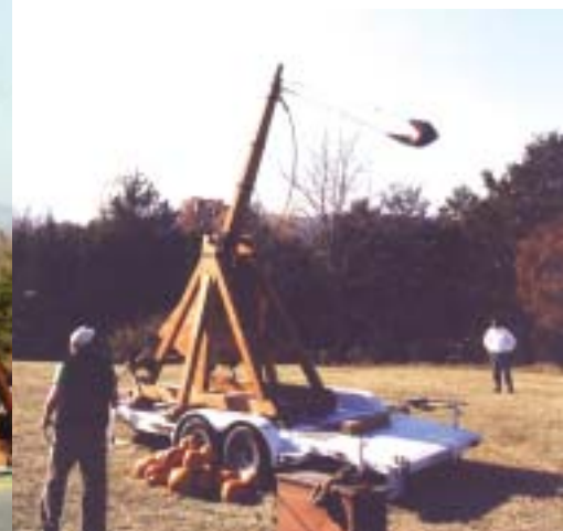
RIGHT TO LEFT: The stages during the launching of a trebuchet — a medieval stone-throwing contraption that used the power of a counterweight and gravity to batter down castle walls.
