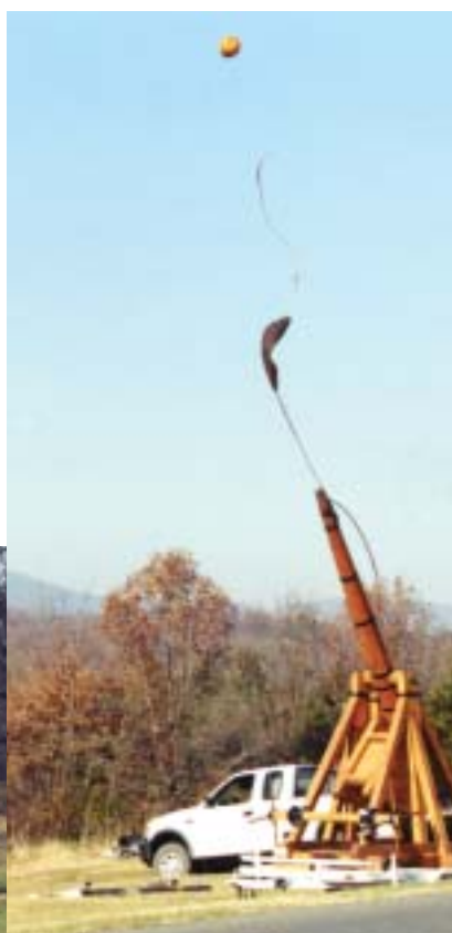
RIGHT TO LEFT: The stages during the launching of a trebuchet — a medieval stone-throwing contraption that used the power of a counterweight and gravity to batter down castle walls.
