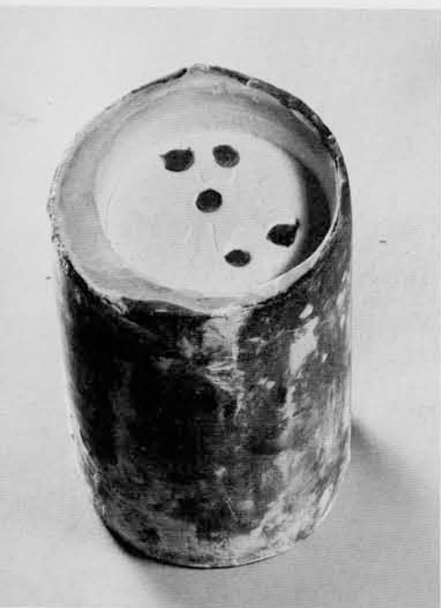
(Left) The wax impression is encased in a fire-resistant clay container (held by a metal cylinder) with the gates showing on top to indicate where the metal will be poured. (Right) The same container in which the wax is replaced by the metal.
