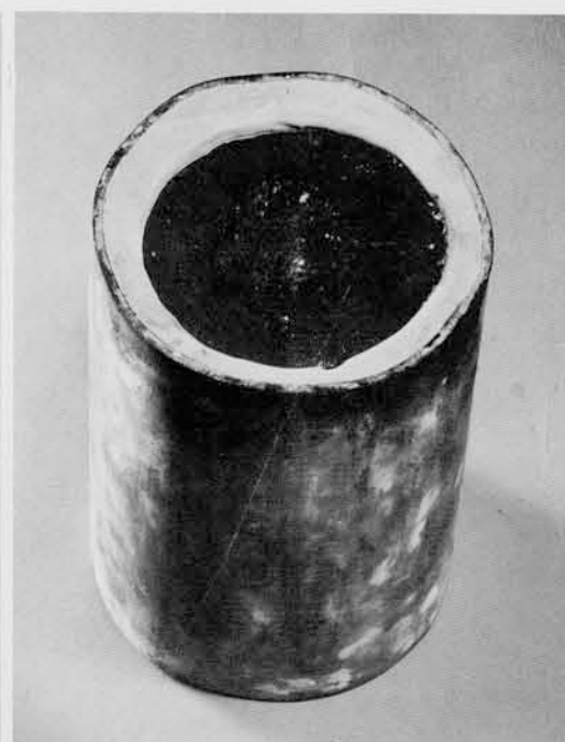
(Left) The wax impression is encased in a fire-resistant clay container (held by a metal cylinder) with the gates showing on top to indicate where the metal will be poured. (Right) The same container in which the wax is replaced by the metal.
