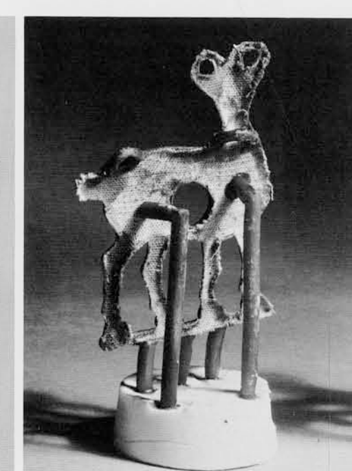
A wax impression with gates attached
