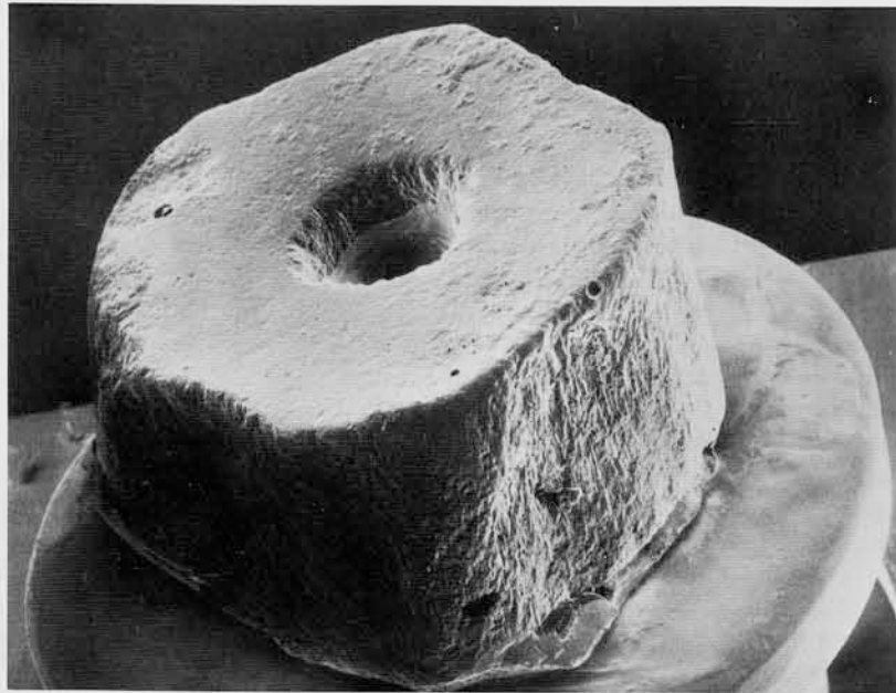
5 Scanning micrograph of a finished, annular bead. The outer surface is relatively smooth and free of scratch marks. Some pitting is present, (x 11).
