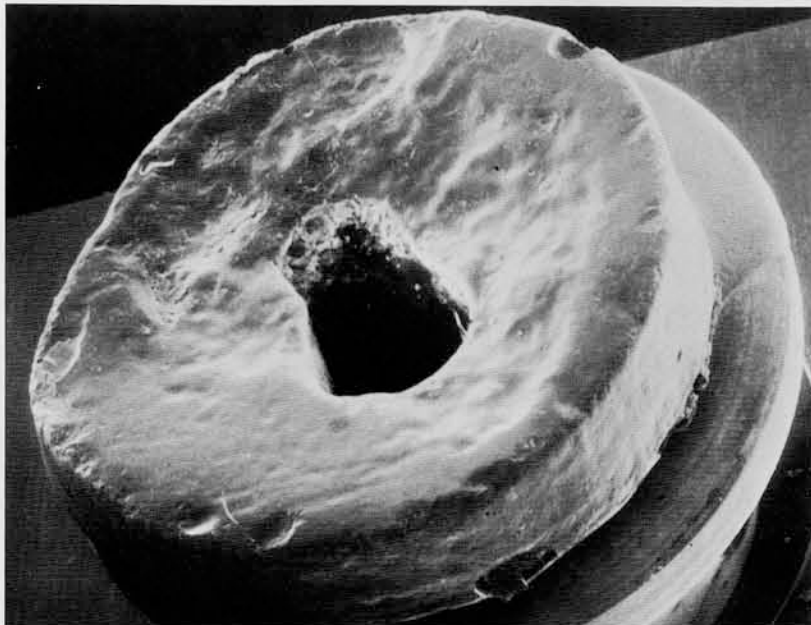
6 Scanning micrograph shows the irregular surface of an annular bead in which the perforation is of an unusual bilobular shape, (x 12).
