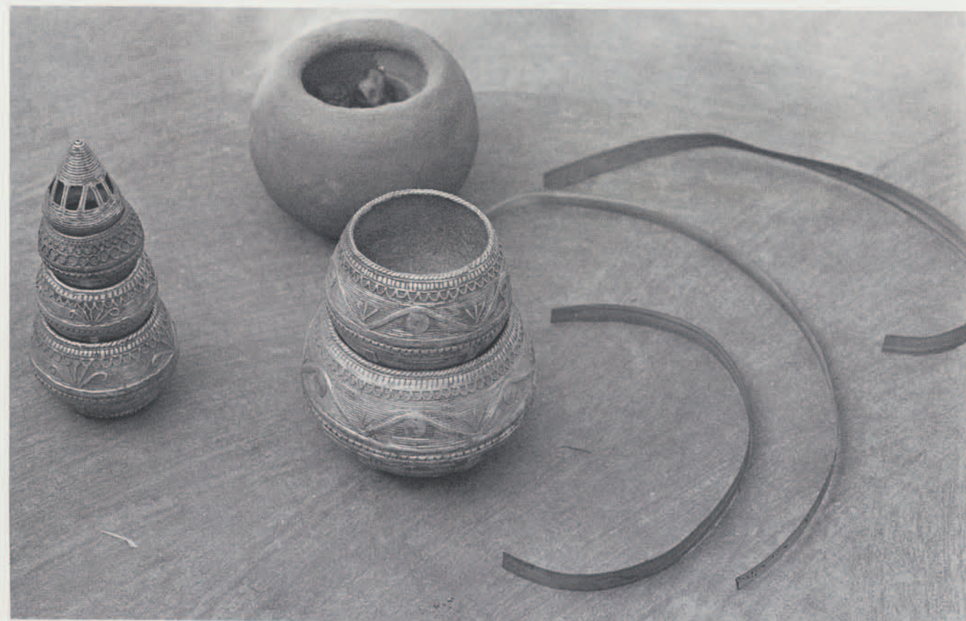
9 Sets of rice measuring bowls are popular with both the traditional and the development market. The bowls are calibrated by wrapping palm leaf strips about the circumference of the sun-dried clay core and filing the core to size.
