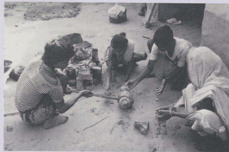
7 A mold just out of the kiln is tipped so that the molten metal in one end can pour into the hollow impression in the other. Fellow artisans watch closely, ready to slap mud onto cracks through which red-hot metal might escape.
