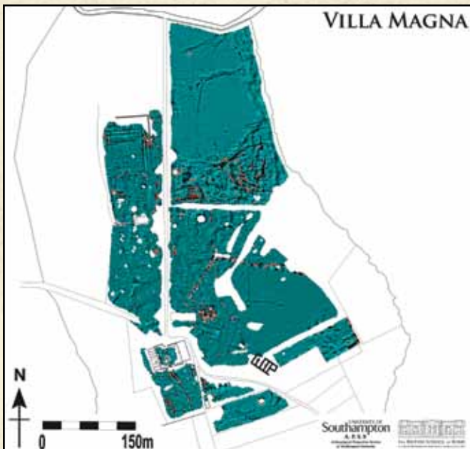
This plot of the magnetometer survey of Villa Magna shows the likely extent and layout of the villa. The red areas indicate areas with high value magnetic anomalies and thus likely walls and other features.
