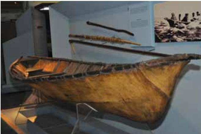
This wooden frame boat is covered with stretched walrus hide coated with seal oil, and dates to the late 19th–early 20th century. Umiaks are still used by Iñupiaq people for hunting whales and for summer transport. (Object #29-47-5, collected by William B. Van Valin)
