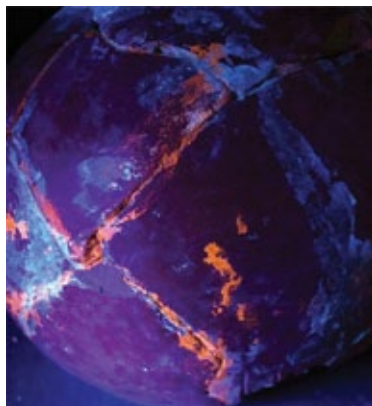
LEFT: The side of vessel #69-35-36 is pictured in UV showing shellac, which appears orange, and cellulose nitrate, which appears white/blue. RIGHT: The FTIR spectrum of one of the adhesive samples (below) matches a known spectrum for shellac (above).
