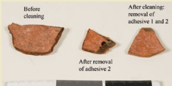
Fragments of the jug are shown representing each stage of cleaning under normal illumination (left) and under UV radiation (right). The UV images show the presence of two adhesives on the uncleaned fragment: an adhesive with yellow green fluorescence (adhesive 2) over an adhesive with orange fluorescence characteristic of shellac (adhesive 1).
