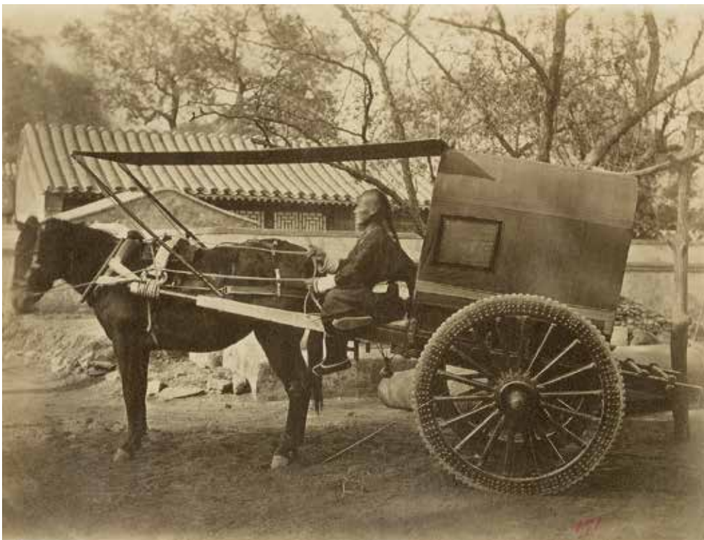
LEFT: Peking (Beijing) Carriage. Mounted albumen print No. 171, ca. 1875–1877. “As distances are great, it is as well to take a cab, of which we see many hundreds in the streets. It is just a box on wheels, without springs, covered on top with a wooden framework, over which is stretched blue shirting; the wheels are very heavy.” PM image 298954.
