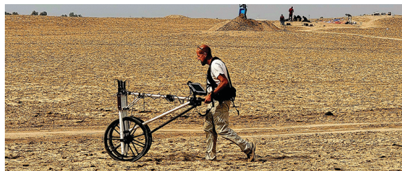
The Lagash Archaeological Project introduced new technology to a dig site last excavated long before smart phones and laptops. Top: a magnetogram of Area H collected in 2019 and 2022. Bottom: Paul Zimmerman operates a rolling magnetometry device, which captures features beneath the surface through magnetic signals that help the team anticipate what excavation will reveal.
