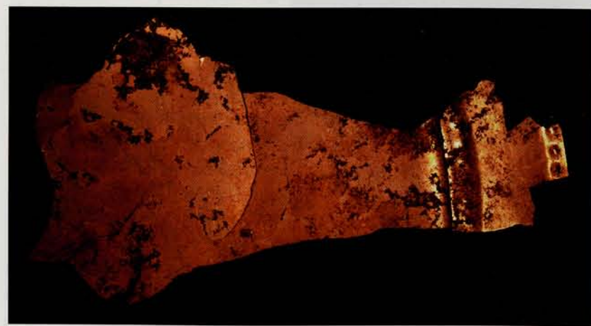
Fig. 1. Fragment of depletion-gilded ornamental disk from Burial 25, Sitio Conte, Panama. Its golden sheen effectively conceals that it is not made of pure gold but of an alloy called tumbaga. This piece has been found to be 75.5% gold, 21.1% copper, and 3.4% silver (a common contaminant of South American gold).
